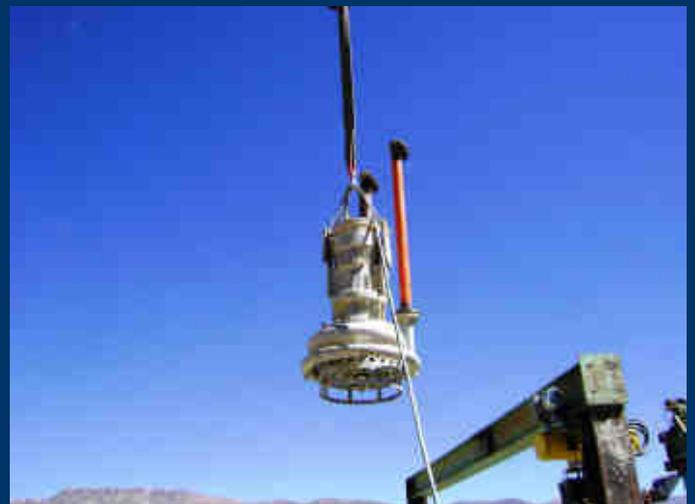
Pond Cleaning – Dragflow EI35 With High Pressure Water Jet Ring
