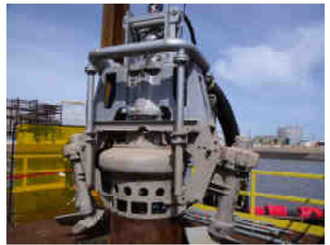
**\Dragflow Pump HY400 and Power Pack – Dragflow Dredge DRH400**
