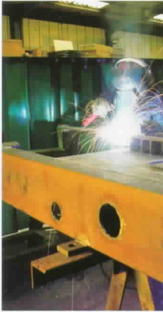
Fabrication of substantial propulsion unit chassis.
