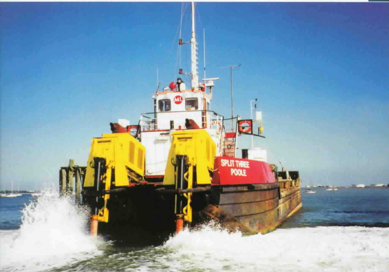
1000 ton split hopper barge with two 350 HP Hydromasters operated by ML (UK) Ltd
