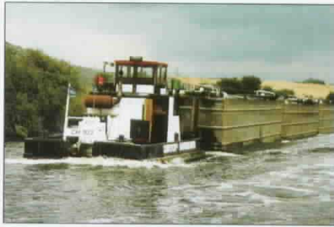
Pusher tug with 700 tonnes load, operating in England's narrow canals. Powered by a single 180 HP unit
