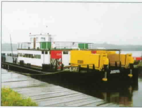
Twin 350 HP Hydromasters powering the Sandaka ferry at 8 knots in hostile waters
